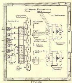
Fig. 141.—Plan view of the railway, synchronous-converter sub-station.
